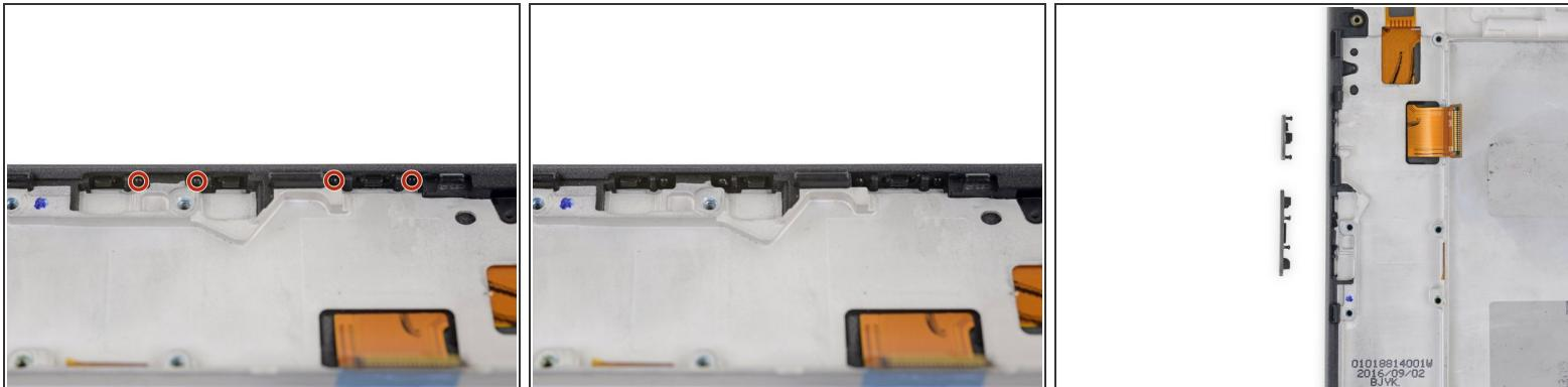
ⓘ The two case buttons (power and volume rocker) are each secured with two mushroom-shaped pins.
